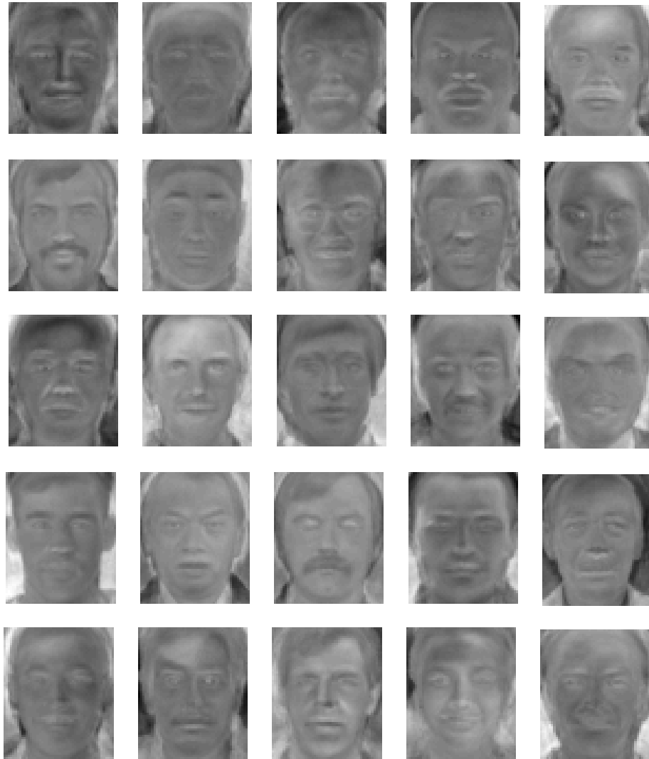
Figure 3.12. Basis images for the ICA factorial representation (columns of A = W_I^{-1} ) obtained with Architecture 2. (See Figure 3.10).
