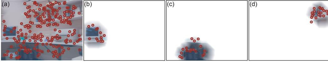
Fig. 2. Example for SIFT keypoints used for object recognition by Lowe’s algorithm. (a) keypoints of the entire image; (b-d) keypoints extracted for the three most salient regions, representing “monitor”, “computer”, and “set of books”. Restricting the keypoints to a region that is likely to contain an object enables the recognition algorithm to subsequently learn and recognize multiple objects.
