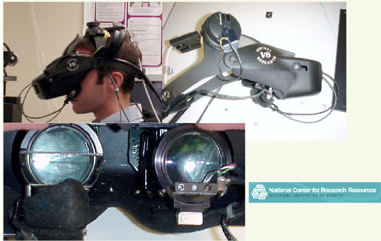
Fig. 8. The head mounted display worn by human subjects has eye tracking capability so that gaze can be tracked in virtual environments.)
