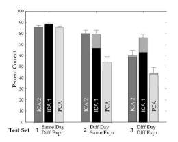
Figure 8. Face recognition performance on the FERET database. ICA architectures I and II are compared to PCA (eigenfaces). Gray bars show improvement in performance following class-specific subselection of basis dimensions. Reprinted with permission from [9]. © 2002 IEEE.
