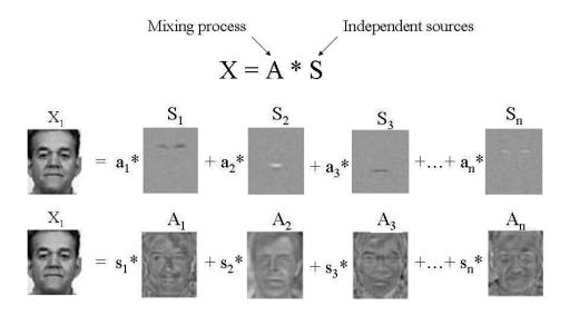
Figure 7. Image synthesis model for the two architectures. The ICA model decomposes images as X=AS, where A is a mixing matrix and S is a matrix of independent sources. In Architecture I (top), the independent sources S are basis images and A contains the coefficients, whereas in Architecture II (bottom) the independent sources S are face codes (the coefficients) and A contains the basis images.
