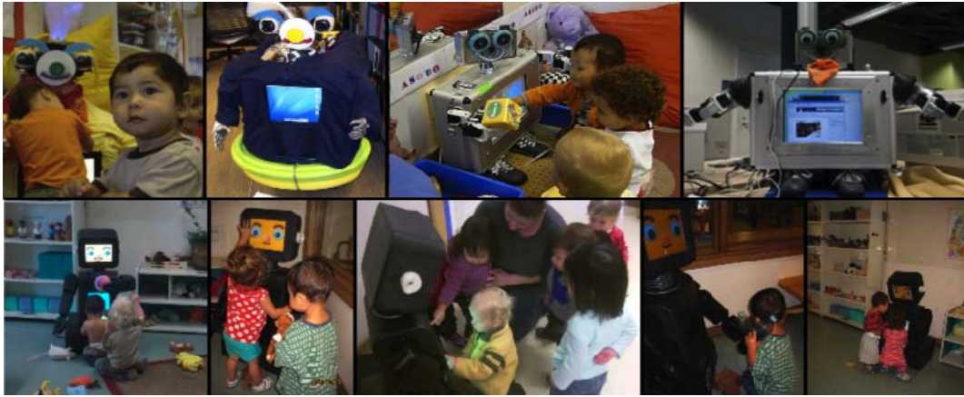
Figure 1. Top row: RUBI progression: from left to right RUBI-1, RUBI-2, RUBI-3 & RUBI-4. RUBI-1 and 2 were remotely operated. RUBI-3 was the first fully autonomous design. Bottom row: RUBI-5 playing with kids at ECEC classroom 2A.
