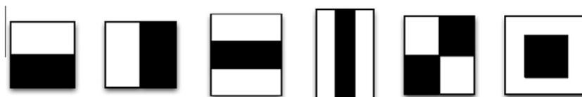
Fig. 4. The six box-filter kernels used for medium time scale temporal modeling. These box-filters compute local frequency and temporal derivatives when applied to low-level feature maps (see Section 2.1)
