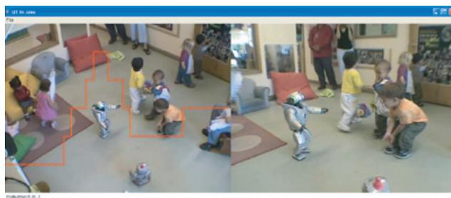
Figure 8: Judges used the keyboard to continuously assign labels to the observed videos representing the goodness of interaction between children and QRIO. Judges can simultaneously see two synchronized movies taken by two cameras are combined into one. The judge can also see the recent history of his/her evaluation which is superimposed on the movie as a red graph.
