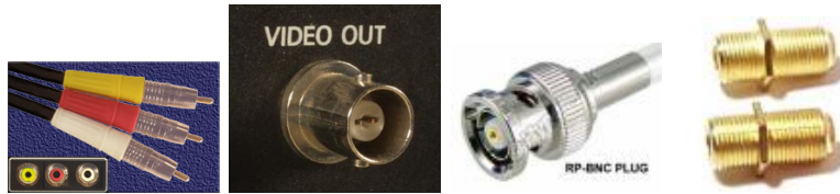
Figure 6: Left: RCA; 2 Center: BNC; Right: F-connectors
