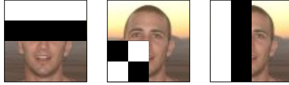
Figure 3.2: Examples of Haar wavelets in a true Haar decomposition superimposed onto a face image. Width, height, and (x, y) positions of all wavelets are aligned at powers of 2.
