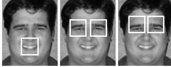
Figure 5.4: The local face regions of the mouth (left), eye (middle), and brow (right) regions from which features were selected for each AU classifier.
