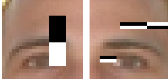
Figure 5.3: Examples of Haar features (selected by Adaboost for AU 1) used for AU classification in our system.
